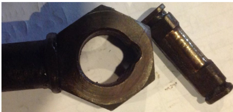
Photo 5: Well-worn “nut” on the Tie-Rod Eye and well-worn Knife Edge. Both items are due for immediate replacement. Don't attempt to repair them!
