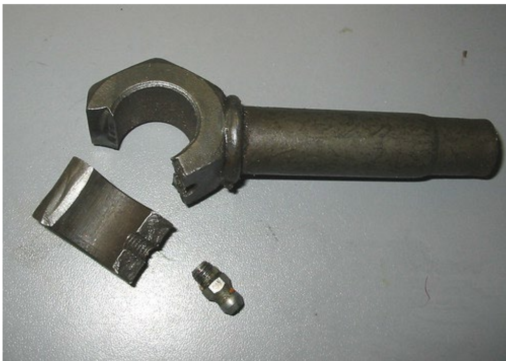
Photo 7: Suspension Tie-Rod Eye destroyed by a modification to fit a grease nipple
