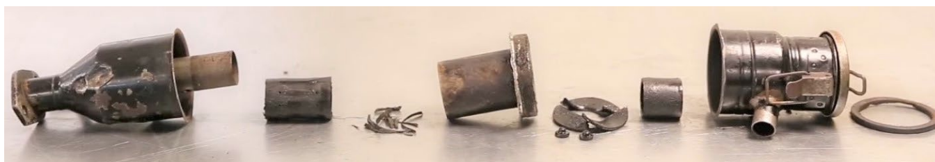
Photo 2. Disassembled 2CV oil breather. Photo courtesy of the Burton Car Company.
