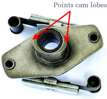
Photo 4 Points cam, springs and centrifugal weights looking from the front, ready for fitting onto camshaft. Note how the springs are fitted.
