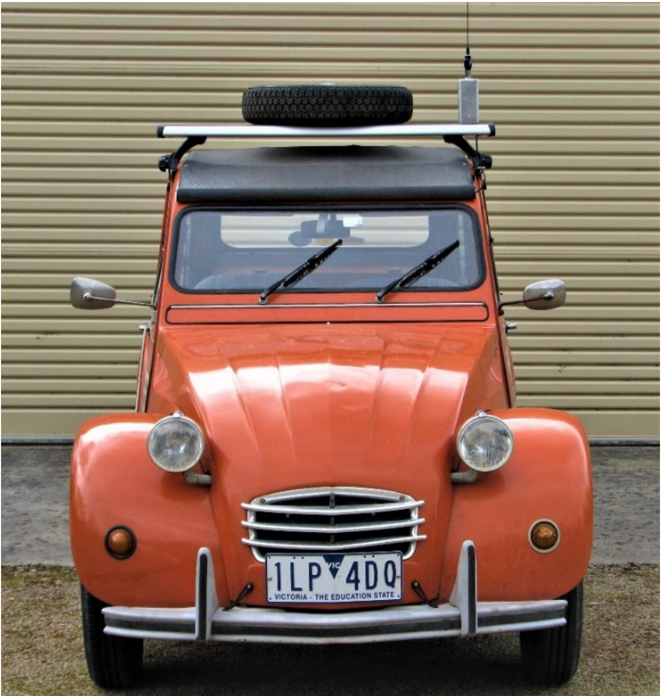
Photo 11 above shows the finished installation on the writer's Raid 2CV. It shows the roof rack, the spare wheel, the metal mount and the antenna, and shows the antenna base being higher than the spare wheel. Job done!
