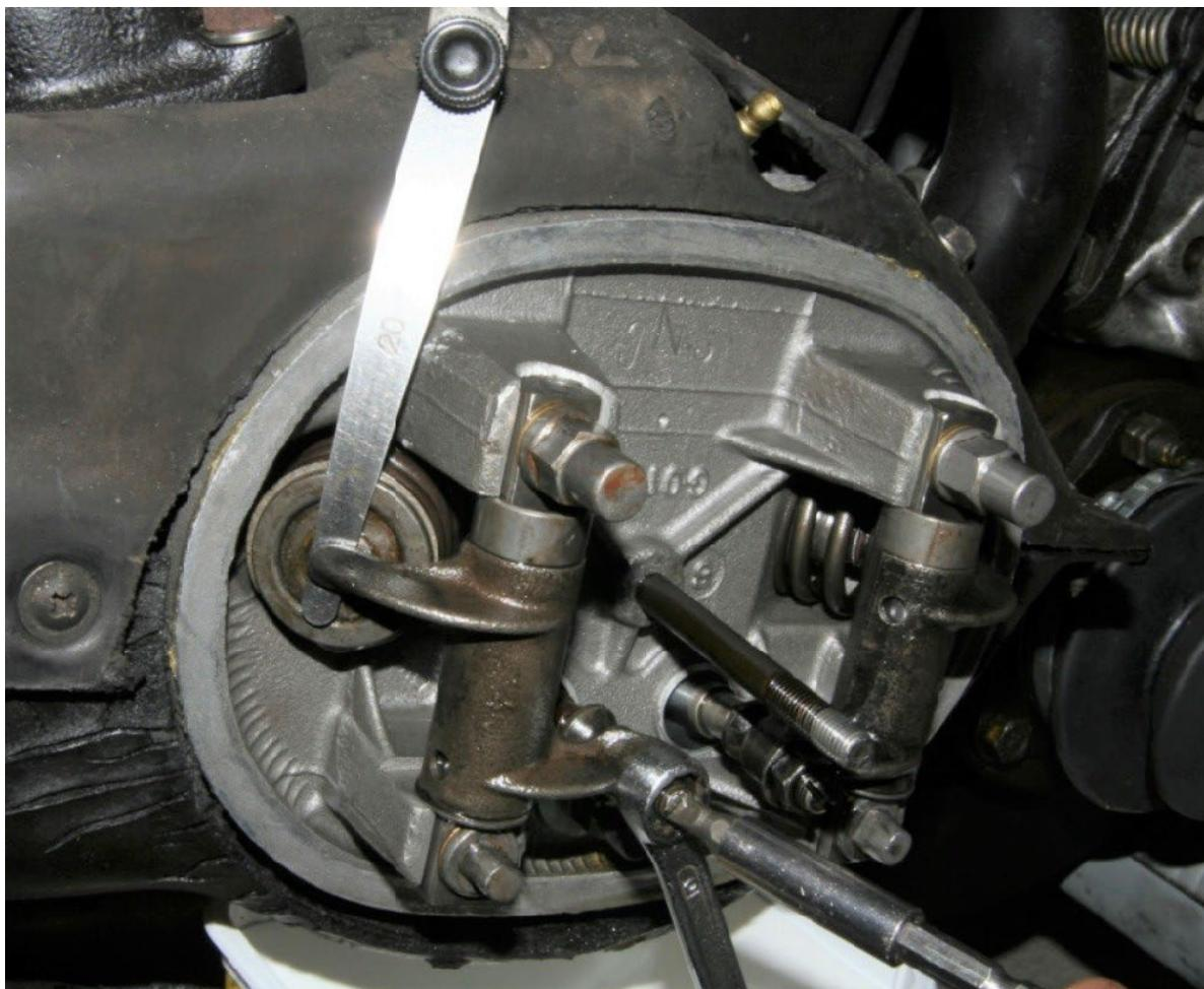
*Adjusting a valve in the 2CV*
