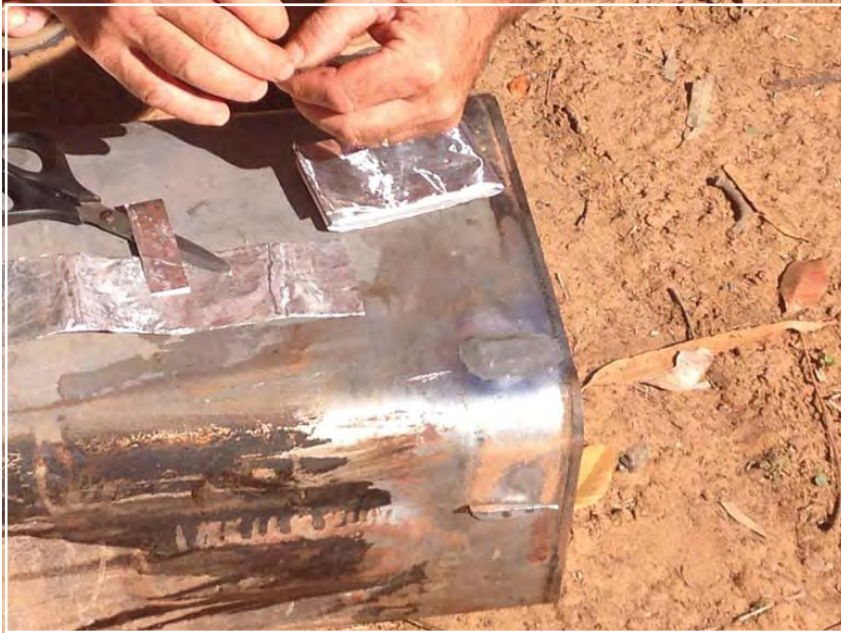
Day 21: The crossing at Roper Bar was only a few inches deep. Stephane's leaking fuel tank was quickly repaired with a metal patch, bonded with soap and Araldite.
