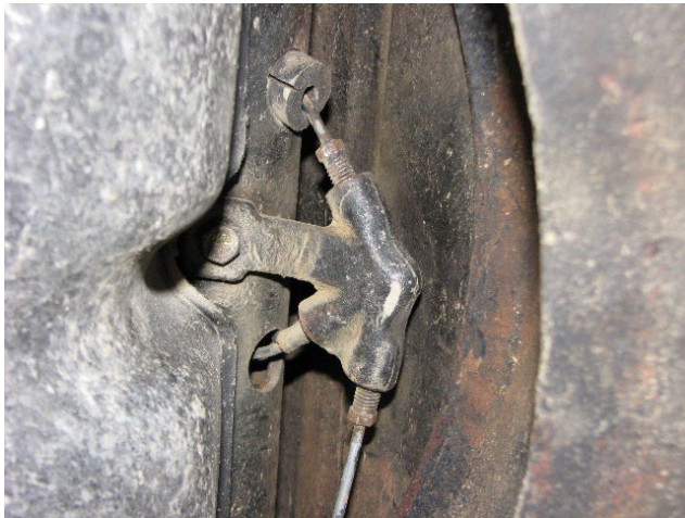
Figure 1 Rear brake line union, next to fuel tank
