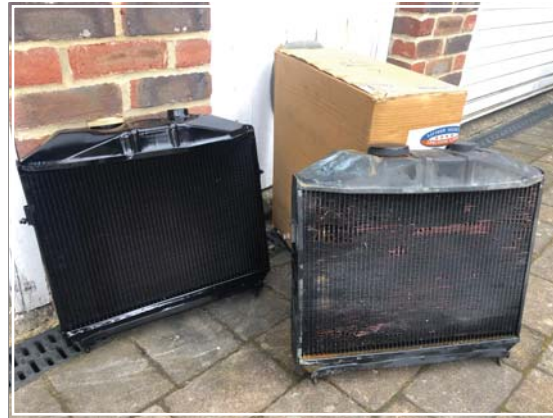
Left: The old and the new radiators. Right: Radiator removal prep. Facing page: ENE ready to head for France.
