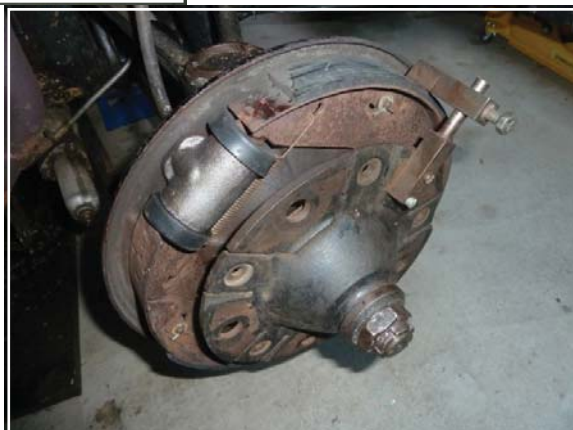
Left: Photos of the dummy drum home-made variant of the ring gauge. Below and facing page top left: Hub with pointer.
