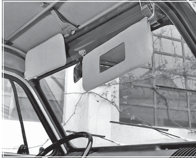
The two sun visors are padded and can also be used laterally. The passenger one is equipped with a courtesy mirror.
