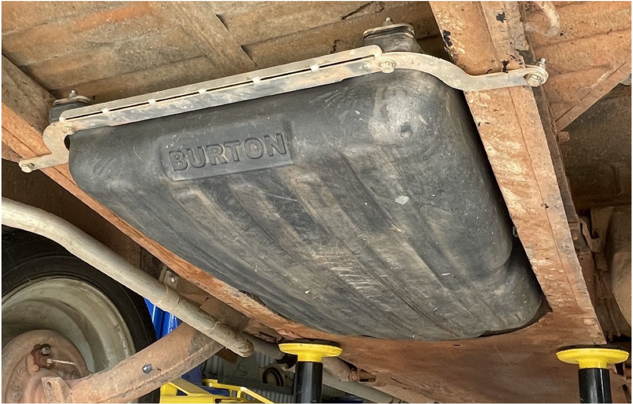
Fig. 2 The 40-litre fuel tank, in the company of some left-over Red Centre dust! Also shown is the tank's rear mounting bracket (supplied with the tank kit).
