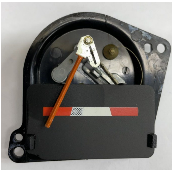
Photo 6. Front of Battery Meter
