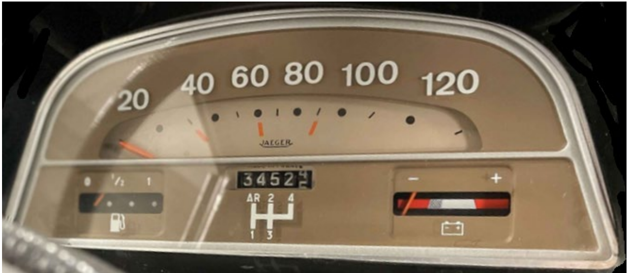
Photo 1. The writer's 1974 2CV speedometer assembly showing the fuel gauge at lower left and the battery meter at lower right.
