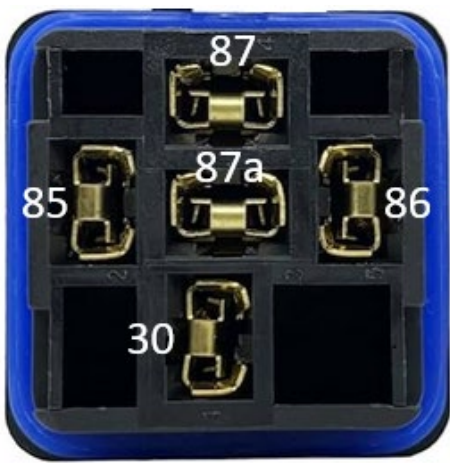
Relay socket numbering from above (looking directly at the sockets from above).
