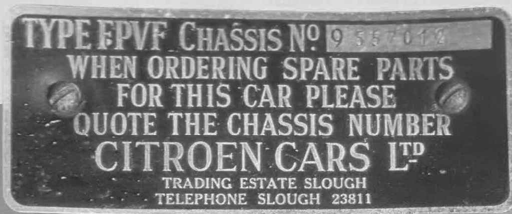
The authentic Slough Works chassis plate, affixed to the engine compartment bulkhead on the left-hand side. (Peter Dulson)
