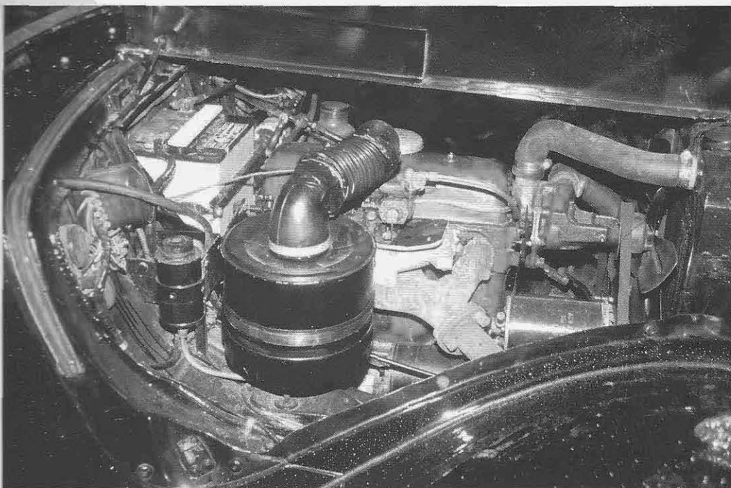
These right and left-hand views of the engine bay show the large oilbath air cleaner fitted to export versions of the Slough-built Traction Avant, and also the tube that conveyed warm air from the radiator to the passenger compartment. This was the only form of heater and demister provided on these cars, although a fan-assisted internal heater was an optional extra. (Peter Dulson)
