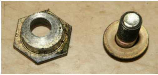
Fig. 2 Eccentric and Eccentric Locking Bolt
