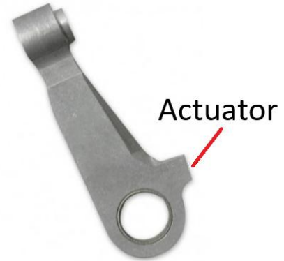
Fig. 5 Actuating arm. The actuator pushes the handbrake pad against the brake disc.
