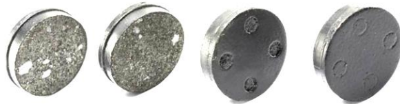
Fig. 4 Set of 2CV handbrake pads. The metal backing plates measure 30 mm in diameter.
